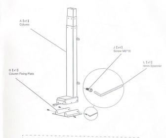
Please fix Lift Column and column fixing plate by Screws M6×16\*4.
